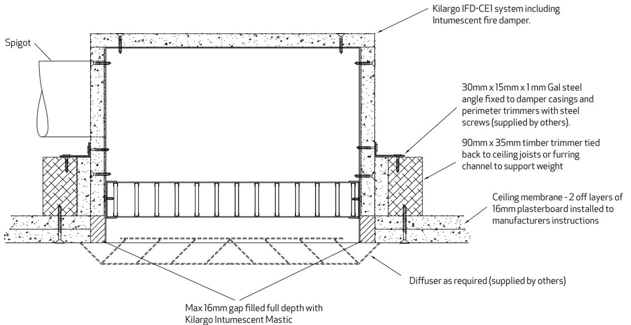
**Supplied as a complete fire-rated enclosure to ensure compliance.**
